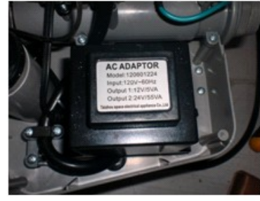
transformer (Double Output)
